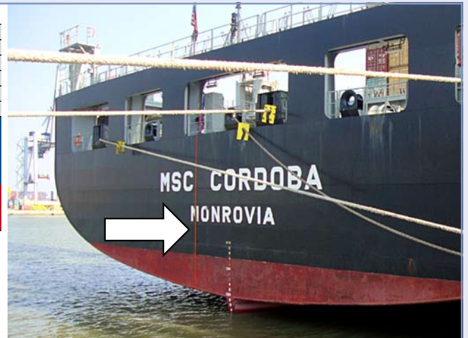
Cable link between camera and control unit on the mooring deck
